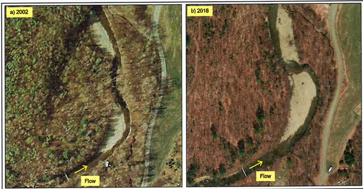
Figure 7. Rapid growth of gravel bar causes meander reformation between a) 2002 and b) 2016 at downstream end of straightened reach at Rollins/Tooker Site.
